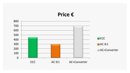
The calculation of the lifetime-cost is based on 4 kW motor IE1 with 40`000 hr lifetime and 10 ct. per kWhr. The 4 kW ACC cost 200€ more as an AC motor and saves 20`0000 kWhr or 2000€ during his lifetime; the payback time is 4000 hr or one year of operation. The value of the saved energy is four times higher as the ACC-sales price.
